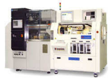
The Tapeless Sawing of QFN 2x2 (2,040 units/strip)
